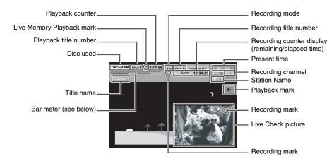
This unit displays the current recording/playback status by the bar meter. (Example of bar meter display)
